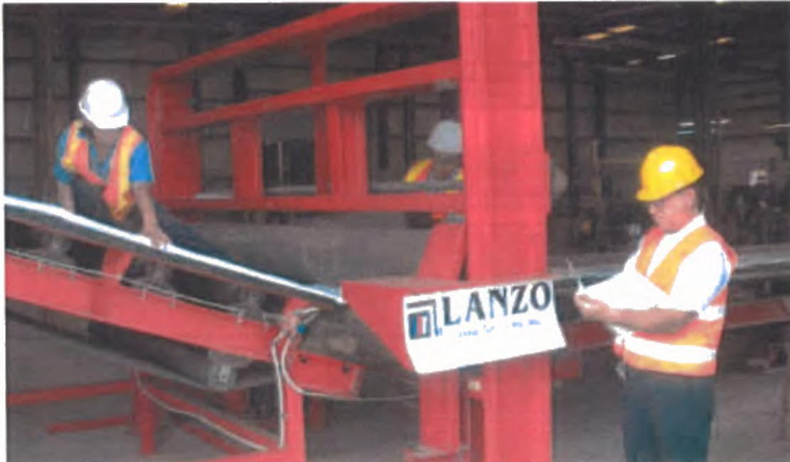
Quality controlled tube impregnation at one of Lanzo Lining Services' state of the art wet out facilities
