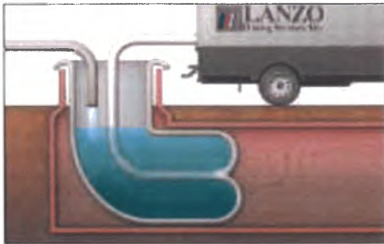
figure 1: Direct inversion installation per ASTM F1216
